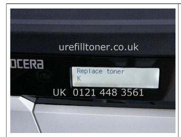
Refill when you get this message on printer LCD panel. As a check, notice that the machine will refuse to print at this point.
