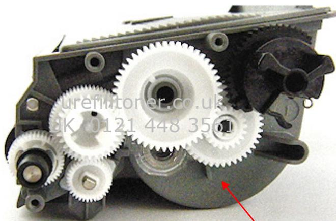
14) Gently separate end plate from cartridge. Avoid displacing cogs. For reference, the correct arrangement of the cartridge's cogs is shown
